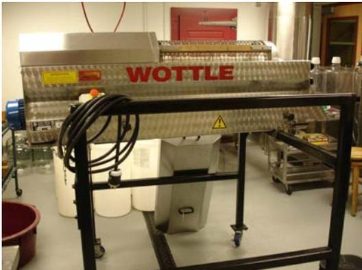
Figure 1. Wottle type-A2 destemmer crusher used for Cabernet Sauvignon berry destemming and crushing
