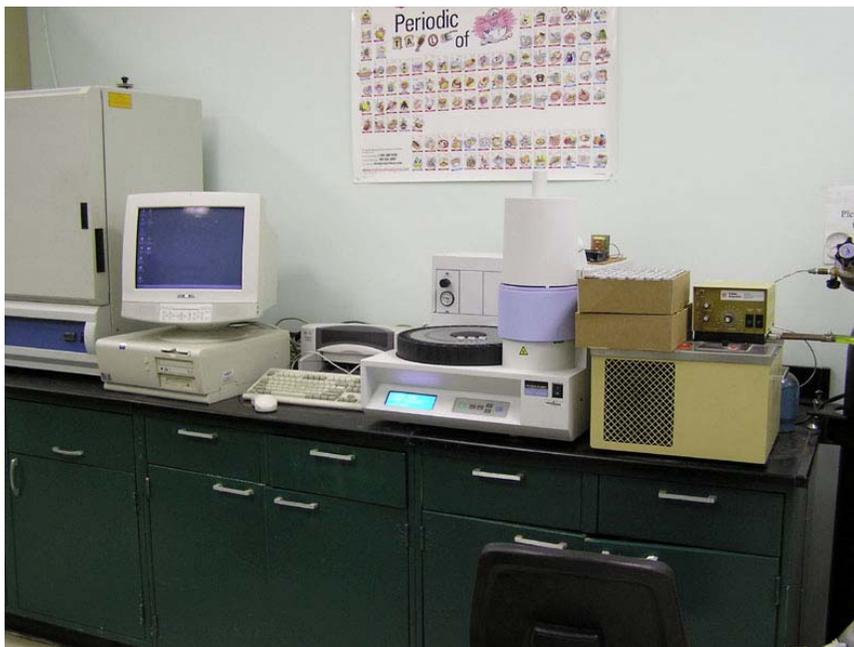
Figure 3. Electronic nose system used for Cabernet Sauvignon analysis
